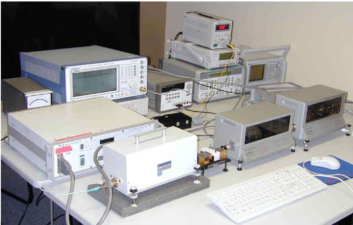
Figure 1: Mixed Harmonic Load Pull setup using: •ATS source tuner and controller •Focus Harmonic load tuner (PHT) and •Focus load Prematching tuner (PMT).
