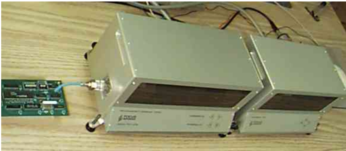
Figure 1 A In-situ@ harmonic load pull testing of mobile phone output power stages.
