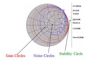
Measurement of the Noise Parameters: The 4 Noise Parameters can be determined if we measure the Noise Figure of a device at a minimum of 4 different source impedances.
