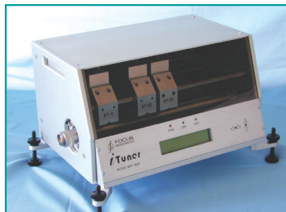
1. The MPT-1840 is an example of the Multi-Purpose Tuner line with three-probe coverage from 4 to 18 GHz that allows impedance tuning at a fundamental frequency and two harmonics simultaneously.
