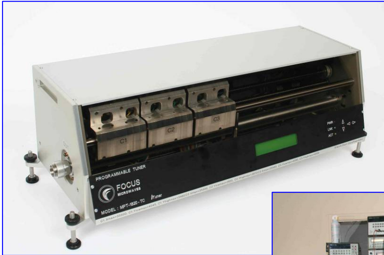
Figure 4: iMPT-1818, 1.8-18GHz for WiMax and WLAN harmonic load pull testing
