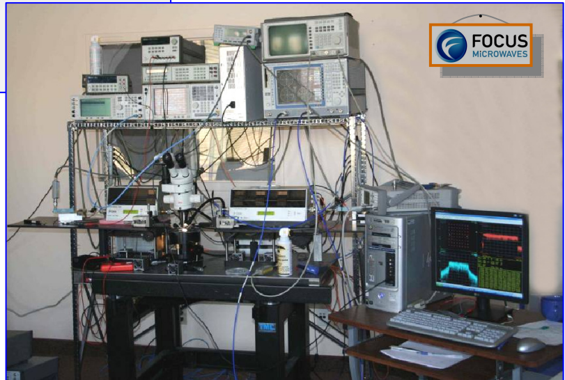
Figure 5: In-house integrated WiMax harmonic load pull setup using MPT multi-harmonic tuner, as per Fig. 3
