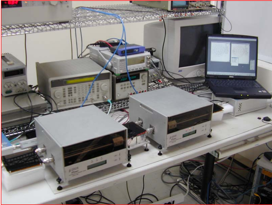
Figure 6: DLPS Setup with a DUT in Test Fixture
