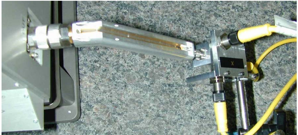
Figure 6: Vibration test at the output of a 45° bend line.
