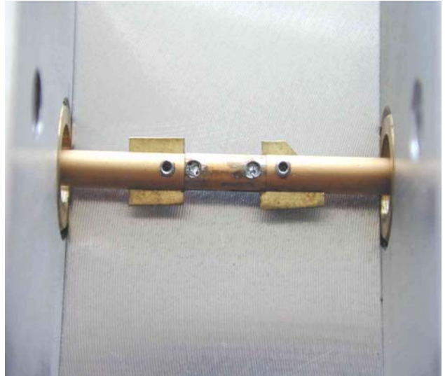
Figure 6: Detail of DELAY standard for package de-embedding.
