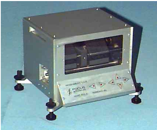
Figure 4: Wideband “Combo” tuner, model 5010-2H with 1.9 mm (V) connectors, f_0=10-50 GHz, 2f_0=20-60 GHz designed for “on-wafer” load pull.
