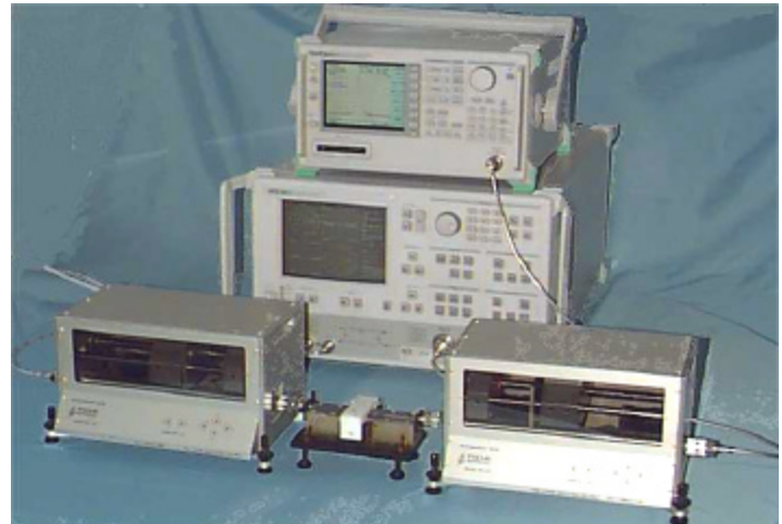
Figures 7,8: Integrated harmonic load pull system (picture shown with test fixture and 1.6 to 18 GHz tuners). Operational up to 44 GHz with 4006-2H tuners.
