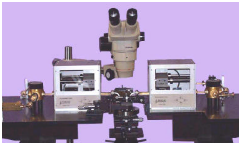
Fig 12: On-wafer Noise tests at 94 GHz using CCMT-11075
