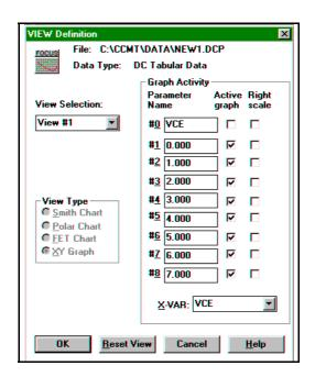
The DC plots can be read out by the mouse. A click on the right button at any given bias point allows to automatically set the DC bias of the transistor to this point through control of an attached GPIB power supply through the load pull measurement software of CCMT or ALPS.
