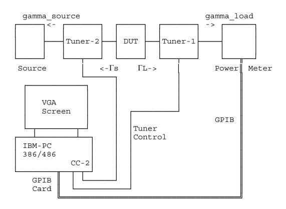
Setup for operating the above example and other Load Pull programmes. CC-2 is the PC insertable tuner controller of Focus Microwaves. DUT = Device Under Test.
