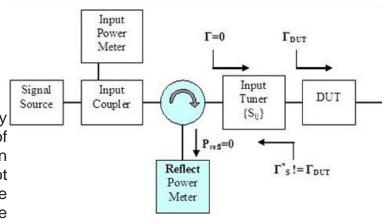
If we use the technique of tuning to minimize the reflected power then the input impedance of the DUT must be calculated from the relation:
