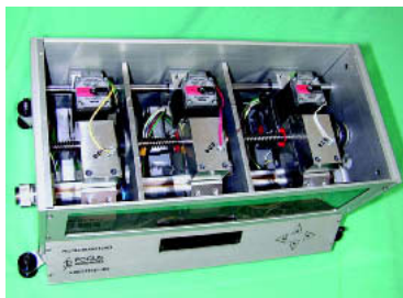
1. The model FST-1818 is a frequency-selective tuner (a) designed for use from 1.8 to 18 GHz, with separate resonators (b) for independent impedance control at a fundamental and two harmonic frequencies.
