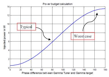
In a typical case the harmonic power requirement will be 10dB above the FET harmonic power (at 2Fo or 3Fo) and in a worst case scenario it will be 15dB above.
