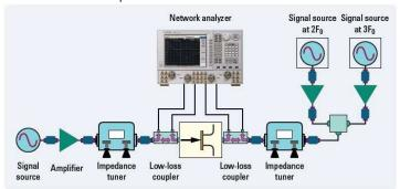
In this setup the load reflection factor  $\Gamma$ -load is created at Fo using the wideband tuner (1) and at 2Fo and 3Fo using additional signal injection from the sources 2Fo and 3Fo, combined with the module (2).
