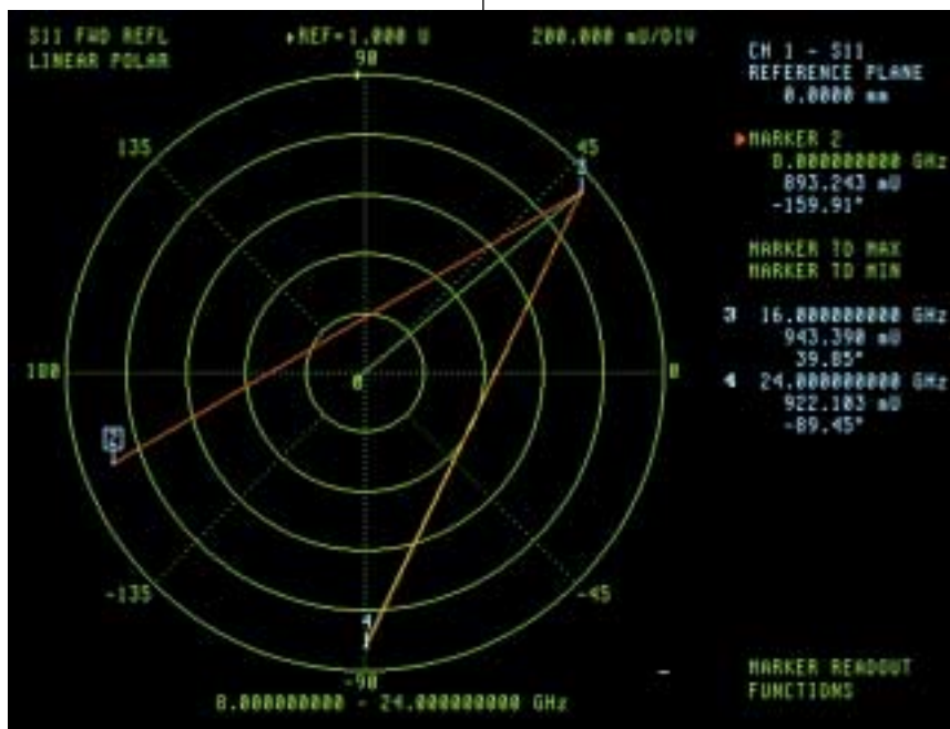
6. This linear polar plot of the 2608-bH combo tuner demonstrates the precise and independent tuning control over the impedances at the harmonic frequencies.
