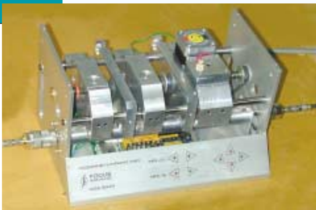
4. This cover-off view of the 1804-bH tuner shows the resonator assemblies and stepper motor used to control a wide range of impedances at the fundamental, second-harmonic, and third-harmonic frequencies.
