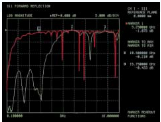
5. The measured S_{11} performance of the 1804-bH biharmonic combo tuner shows the low-loss performance of the instrument.
