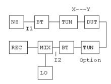
Noise Temperature Tn: Is the temperature (in Degrees Kelvin) of a resistance connected at the input of the device, that will generate as much noise power at the output of the device as the device itself.
