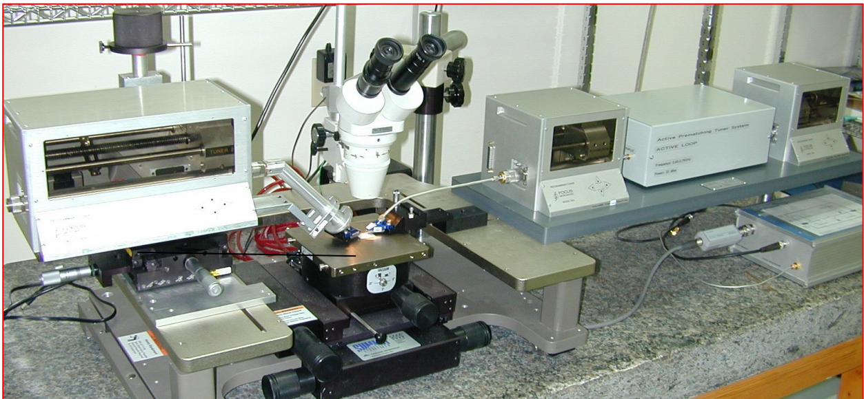
Figure 1: On wafer set-up using passive tuners and \Gamma_{Load} enhancing active power section
