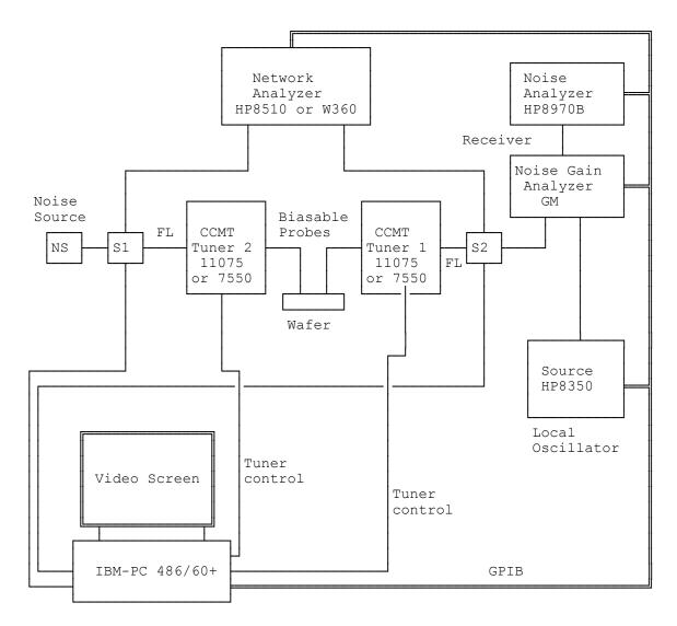
Legend: NS = Waveguide Noise Source (Millitech or Noisecom)
