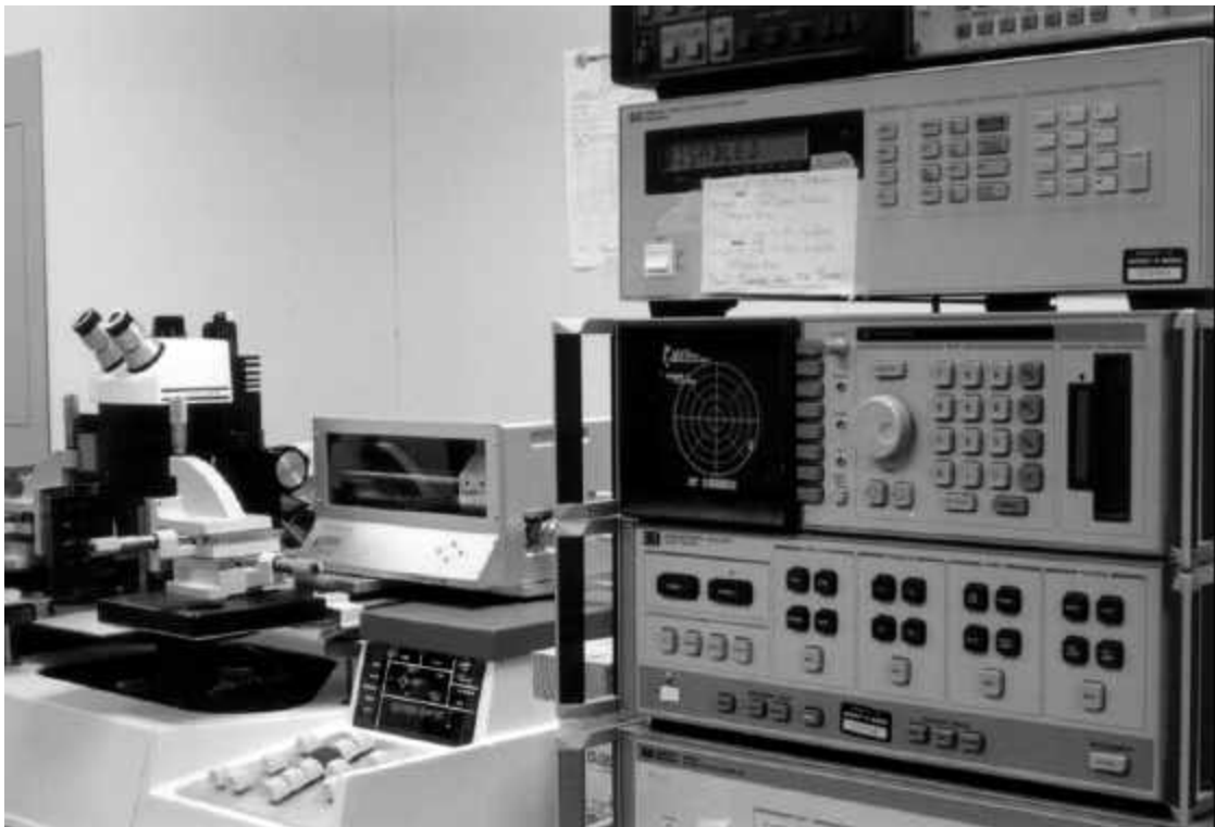
Figure 15: On-Wafer Measurement Setup 0.8-18 GHz
