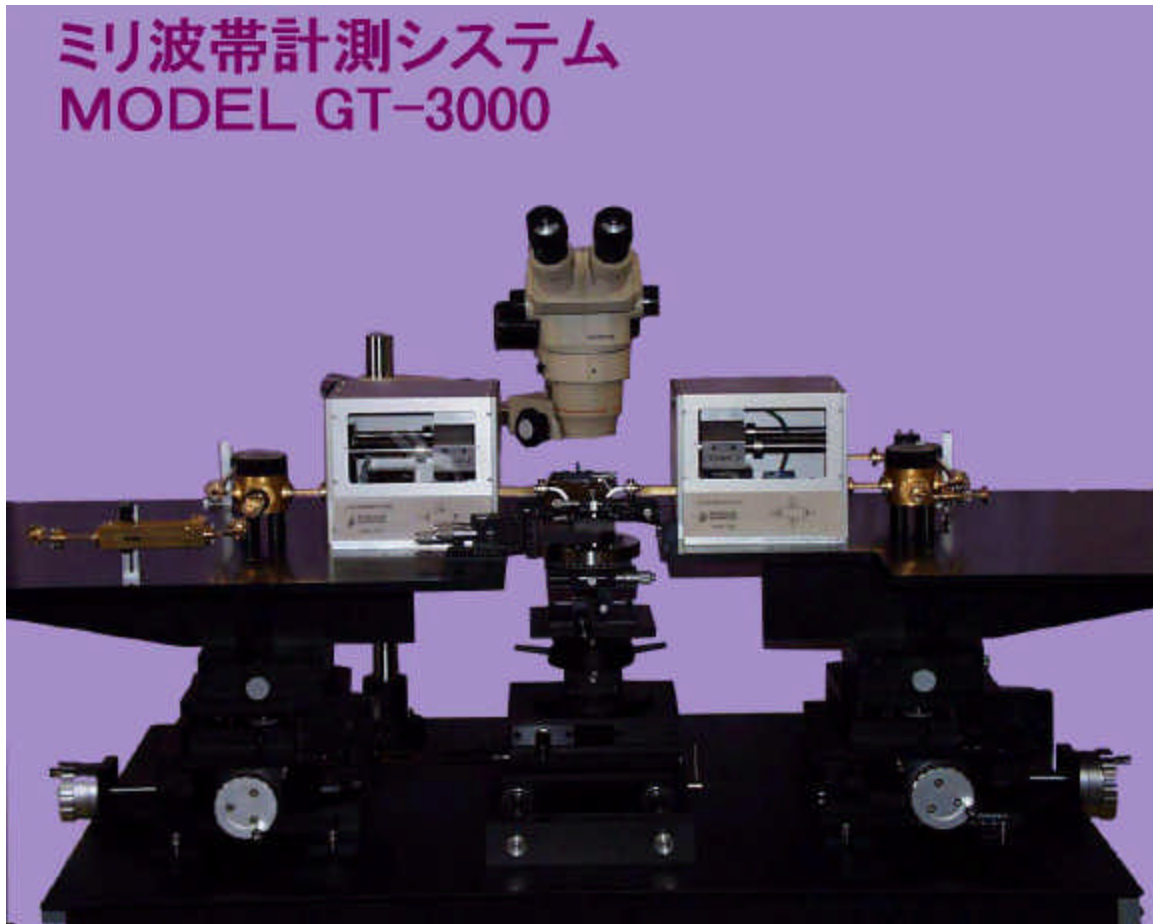
Figure 14: Millimeterwave On-Wafer Noise Measurement Setup
