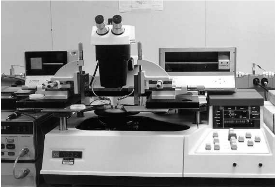
Figure 4: Setup for Noise and Load-Pull measurements
