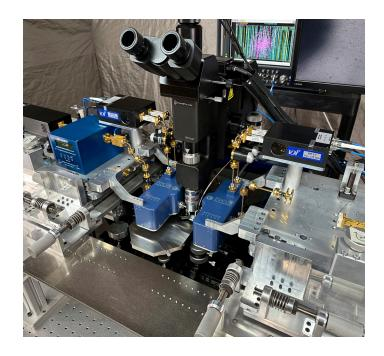
The extreme low-loss RF probes used in the waveguide tuners are meticulously engineered to achieve optimal tuning accuracy and repeatability. These probes are designed to be free of spurious resonances, ensuring that the signal integrity is maintained throughout the tuning process. This high level of precision is crucial for applications that demand exceptional performance and reliability.
