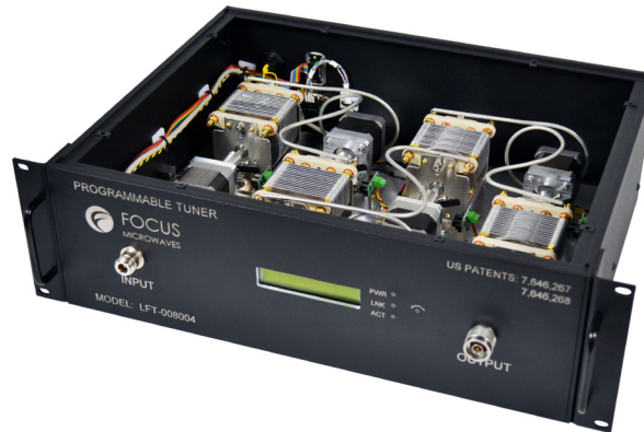
Figure 2: Inside view of a 4 section LFT
