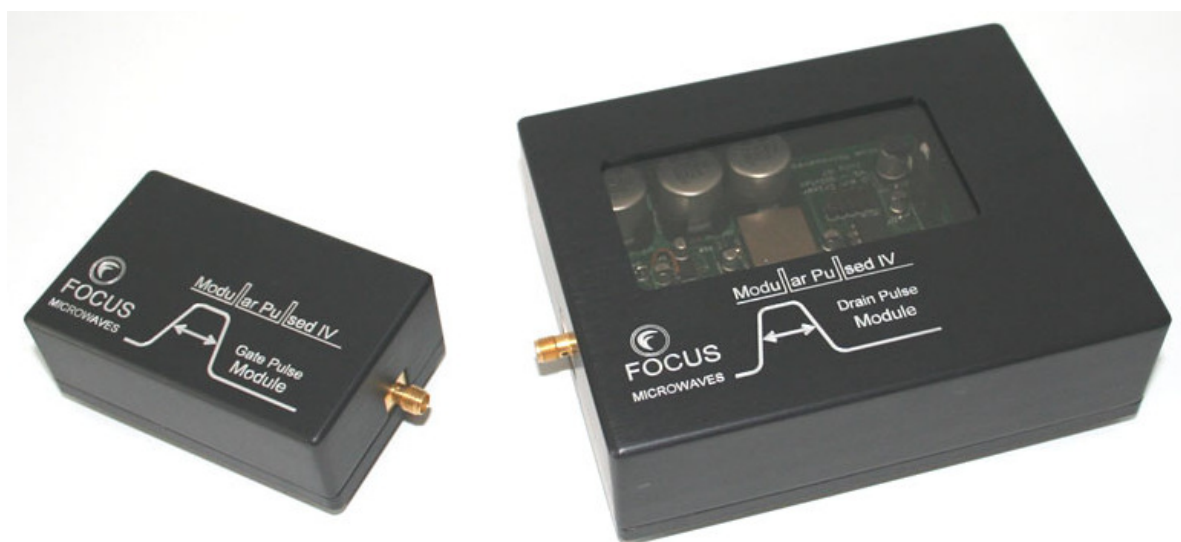
Figure 2: Gate and Drain Pulse Module of the MPIV
