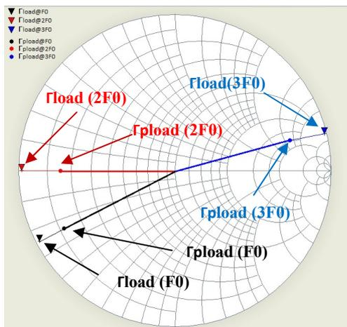
Fig. 2: Hybrid Impedance Synthesis ( $\Gamma_{load}$  and  $\Gamma_{pload}$ )
