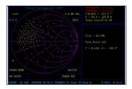
A **Section** is a rectangular zone of the Smith Chart that includes only tuner calibration points.
